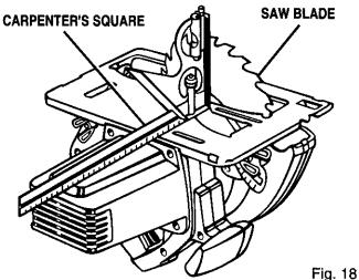
Your saw has a positive 0° bevel stop, that has been factory adjusted to assure 0° angle of your saw blade when making 90° cuts. However, misalignment can occur during shipping.
